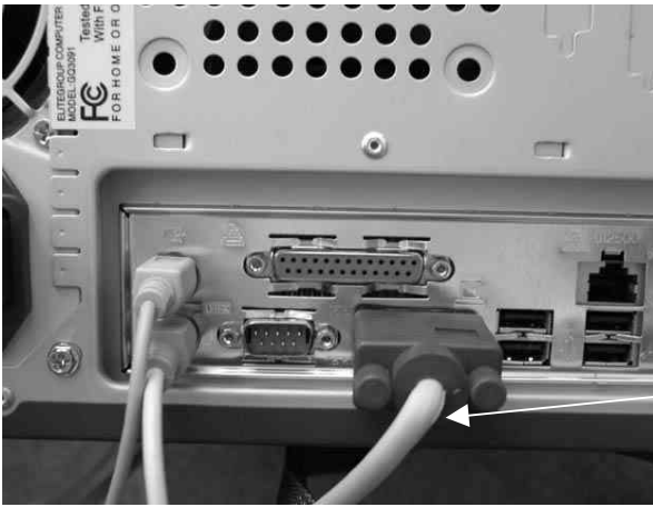
VGA Cable to Monitor
